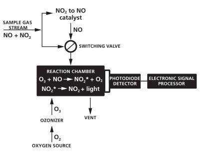
The analyzer can also convert the NO<sub>2</sub> in the gas stream to NO, which is then passed to the O<sub>3</sub> reaction chamber, resulting in the total NOx value that was present, allowing the analyzer to speciate the concentrations of NO, NO<sub>2</sub> and total NOx with the same analyzer.
